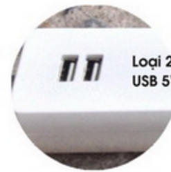
Type 2 USB charging port 5V-1A
